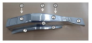
By determining the processing conditions, molding without defects (cracks) is possible.
